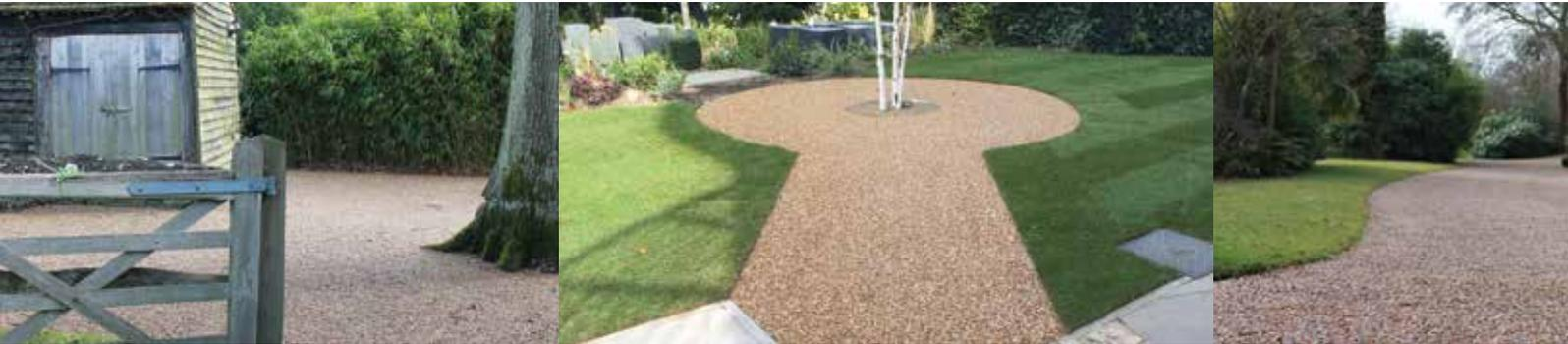
Addagrip Amber is a Resin Bound Surfacing System based on a blend of natural aggregates and a natural oil Aromatic Polyurethane resin where the colour is enhanced in the initial curing process.
