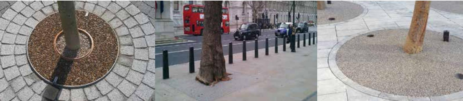
Addagrip TP Resin is normally mixed with a 6-10mm grade of washed, clean and dry aggregate, and laid to create a porous surface. It is ideal for tree pits and light use footpaths.
