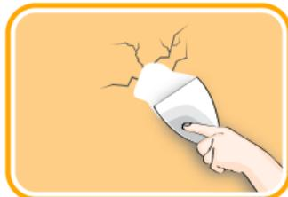
**3)** Apply in layers up to 5mm per coat allowing each layer to dry before overcoating.
