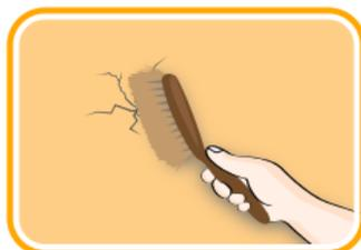
**1)** Ensure surfaces and holes are clean, dry and free from dust and loose material. Prime any exposed nail / screw heads with a suitable metal primer prior to application.
