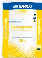
An acrylic based, ready mixed rendering compound used on all common types of interior building surfaces, to level and rectify irregularities up to 10mm in thickness, when applied in multiple coats at a maximum thickness of 5mm per application. It acts as a filler basecoat and will need to be finished off by over coating it with the Sprayplaster finishing products listed below, before painting can commence.
